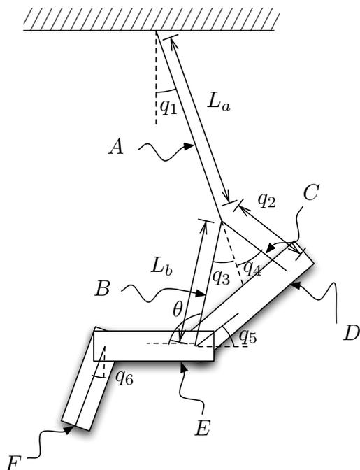
Figure 2: Model of swing showing generalized coordinates and body labels
