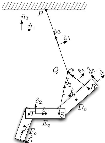
Figure 3: Model of swing with points and axes shown
