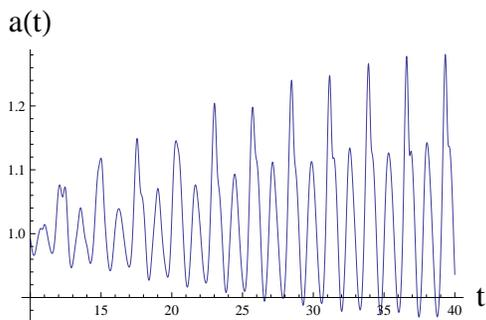
Figure 5: Magnitude of acceleration (units g) over time in case 4 obtained from simulation at point  $E_o$
